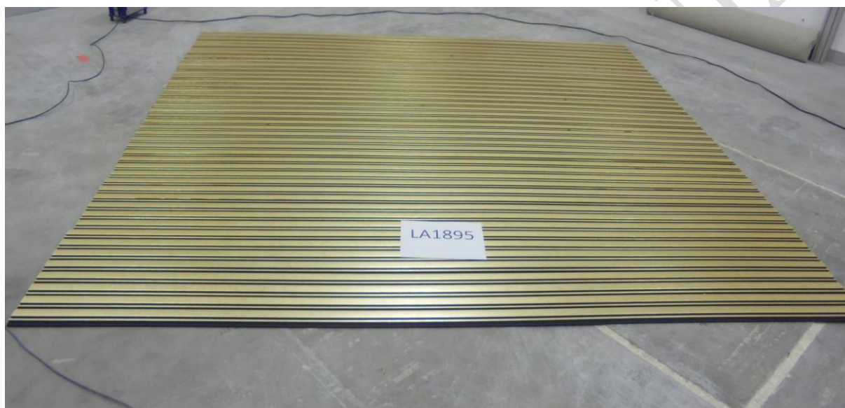
Fig. 2. Test object LA1895 photo LAMELIO wall panels, in reverberation chamber in Vibroacoustic Tests Laboratory in CTO S.A.
