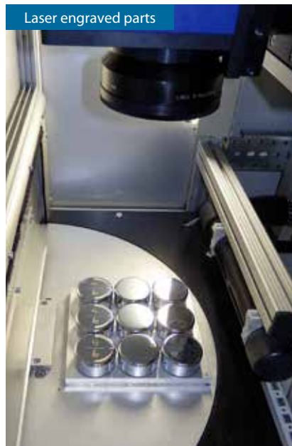
Laser engraving machine Foba Vario RD 15
