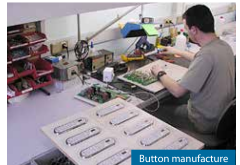
Final and safety inspection of electronic parts
