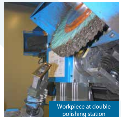
4 workpiece holders each with 2 axes, 1 grinding unit with 2 grinding stations, 2 double polishing units each with 2 polishing stations. All stations 5-axis
